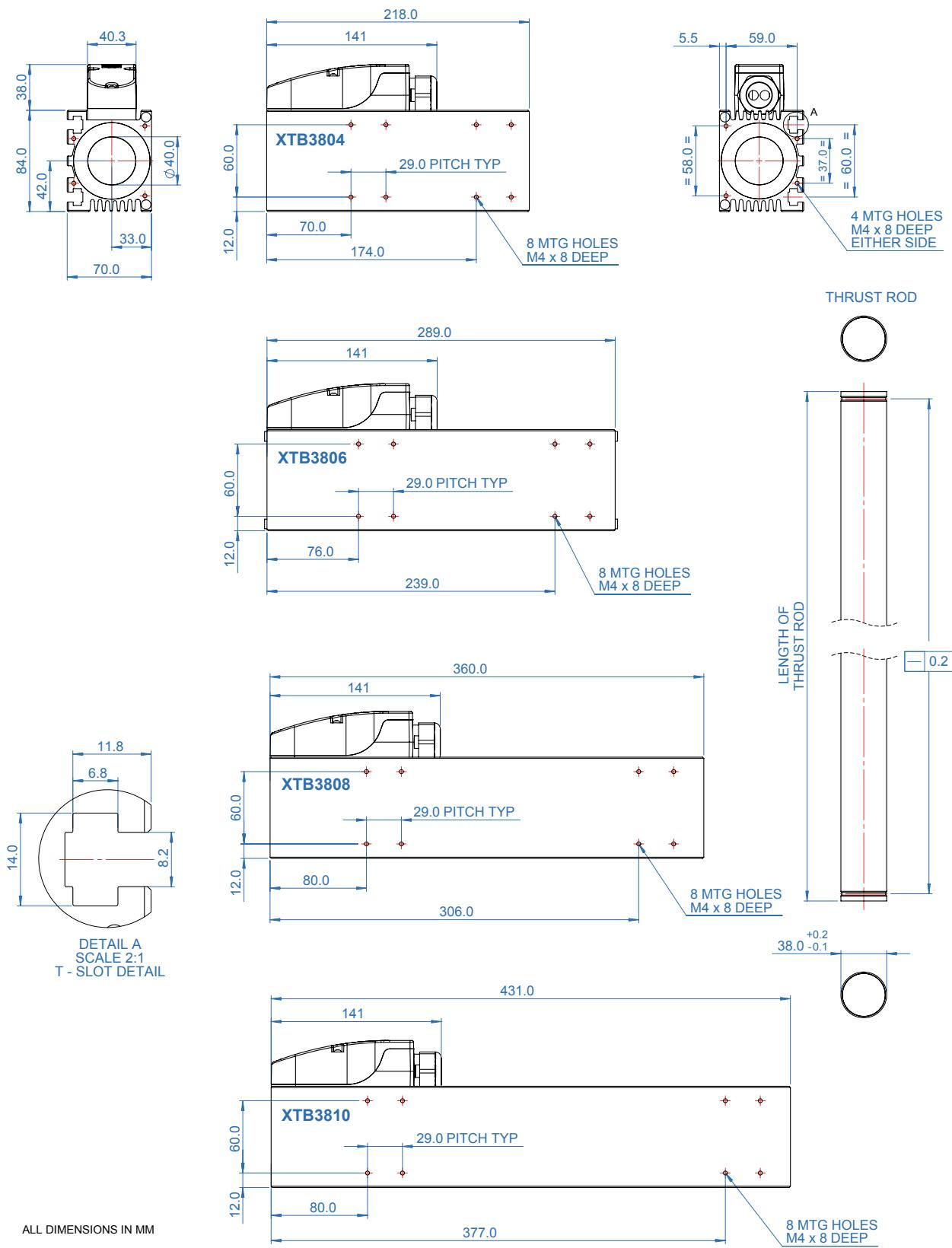
Available thrust rod lengths (dimensions in mm)
